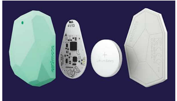
Bluetooth Smart beacon built by Krakow, Poland-based startup Estimote. (Image courtesy of Estimote)
