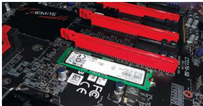
1. Micron's M.2 NVMe module uses an x4 PCI Express interface.
