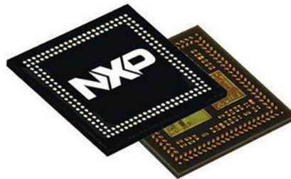
1. NXP's SCM-i.MX 6SX incorporates a 1-GHz Cortex-A9 and an 227 MHz Cortex-M4 in a 13- by 13-mm Package on Package (PoP).
