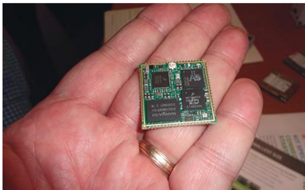
2. Digi International's 29- by 29-mm CoreConnect i.MX6UL has a Cortex-A9 with Bluetooth 4.0 and 802.11a/b/g/n Wi-Fi support.
